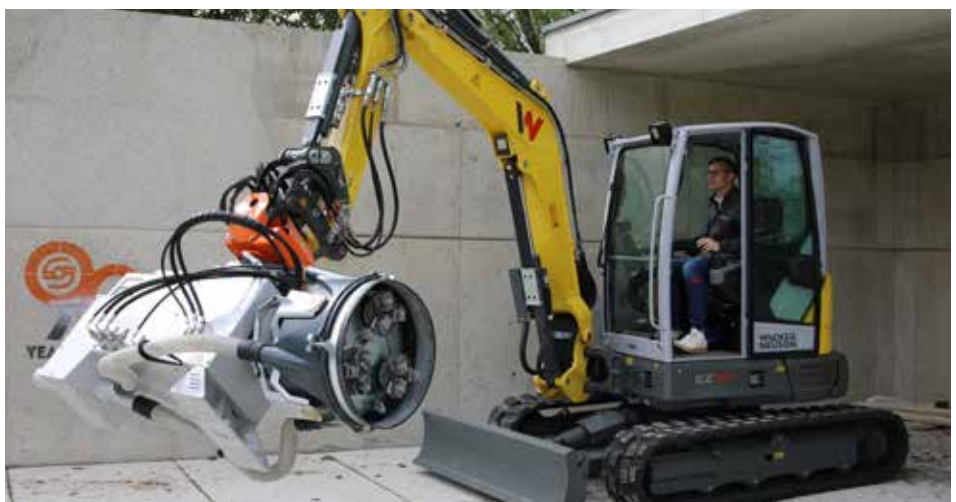
A medium-size excavator equipped with the new WDS 530S concrete grinding attachment.
