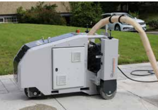
The new BEF 400RC remote controlled milling machine in operation.
