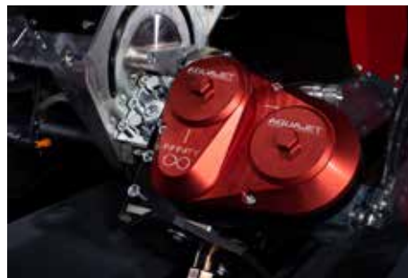
The constant speed and continuous movement of an infinity pattern removes more concrete in a single pass and leaves behind a more consistent result.
