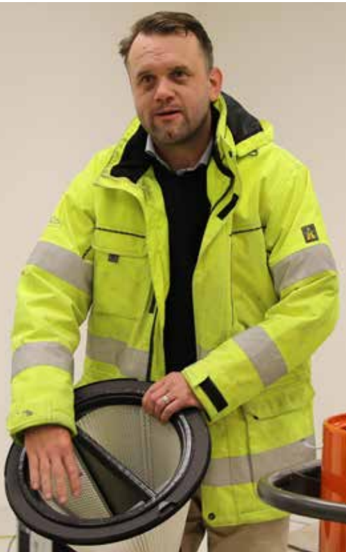
Christian Nyberg shows how the new cone shaped pre-filter is divided into two chambers, making it possible to alternately keep the filter clean during work. This means that the user does not have to interrupt work to clean the filter manually.
