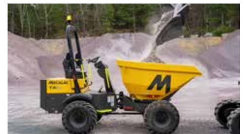
Site dumpers drive productivity because the skip has a capacity double that of the common skid steer bucket.
