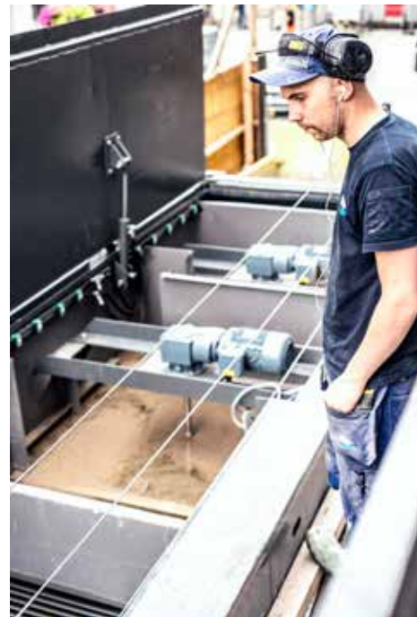
Concrete isn't the only thing that can be recycled. Aquajet's EcoClear neutralizes the pH and reduces suspended solids in blast water, so that it can be reused for the hydrodemolition process.
