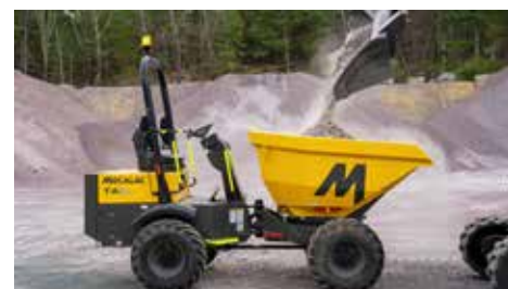
Site dumpers drive productivity because the skip has a capacity double that of the common skid steer bucket.
