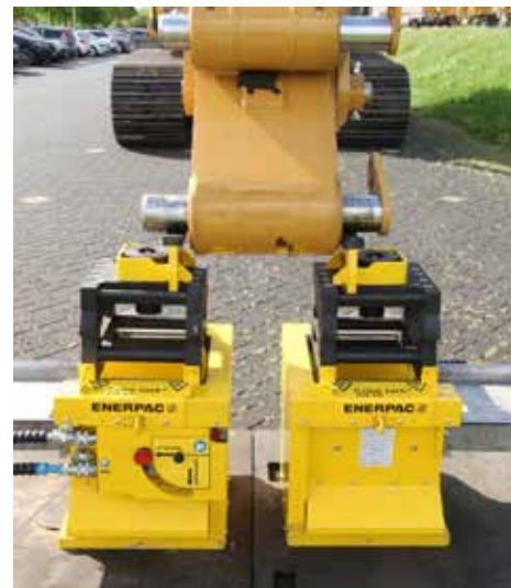
Enerpac cube jacks supporting the excavator boom and arm.
