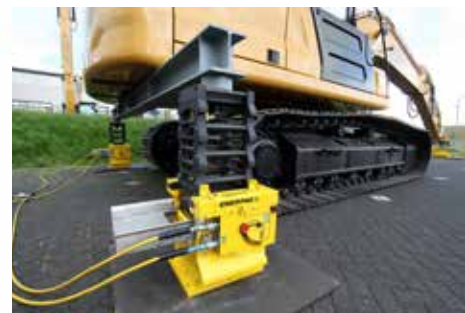
Enerpac cube jacks supporting the excavator cab.
