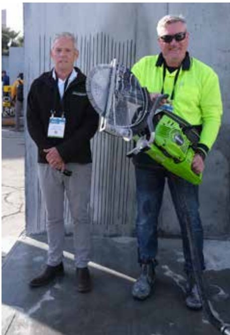
Steve Terpstra and Craig Penty from Australian Guard Systems showed a very innovative system to eliminate both silica dust and fumes when power cutting. A dust extraction system connected to a power cutter takes care of an eliminate both fumes and silica dust from the workplace.
