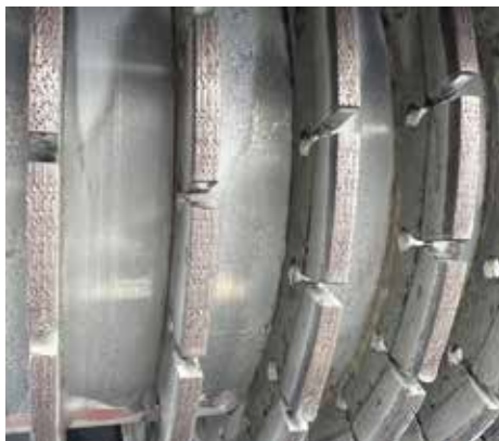
The grinding shaft with diamond saw blades and spacer discs.
