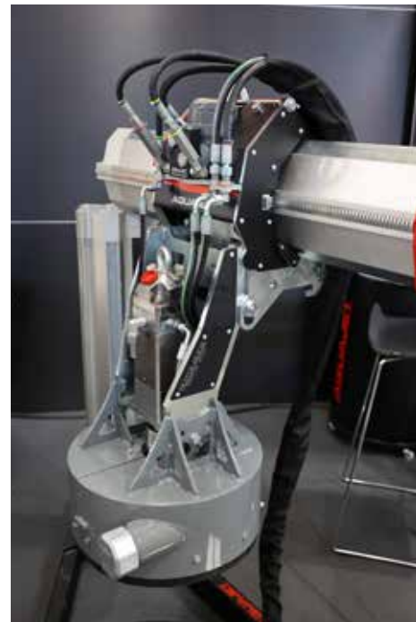
The Rotolance attachment is a powerful surface preparation tool. Contractors can utilize the Rotolance to remove concrete, rubber coatings, paint, rust, plastic, and other materials.
