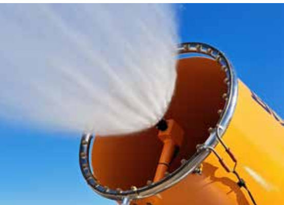
The center nozzle features a variable spray pattern. Photo: BossTek.
