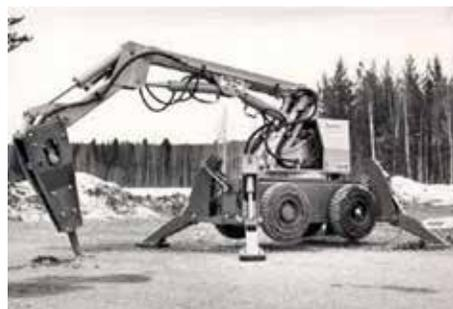
The first serie produced demolition robot and Brokk robot. Copyright: Brokk AB.
