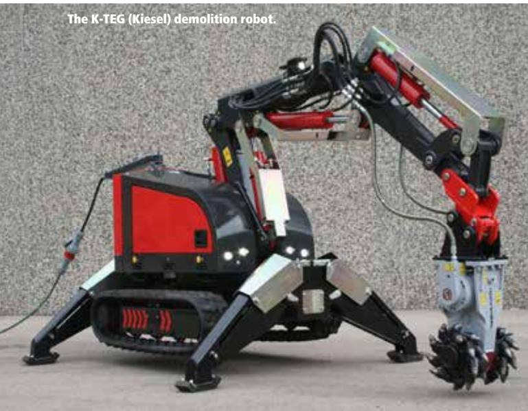
The K-TEG (Kiesel) demolition robot.
