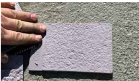
The International Concrete Research Institute identifies Hydrodemolition, also known as water blasting or water jetting, as one of few methods capable of achieving concrete surface profiles 3 through 10.
