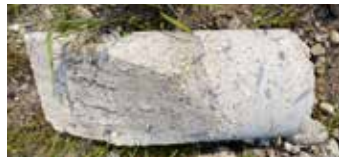
In total, 32 cores with a diameter of 14 in (350mm) had to be drilled for the installation of the docking poles.
