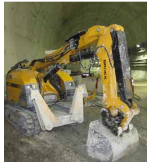
In addition to replacing large crews with handheld equipment, remote-controlled demolition machines with the right attachments can also do the job of several common compact machines — including skid steers and mini excavators — allowing contractors to increase productivity without increasing their fleet.
