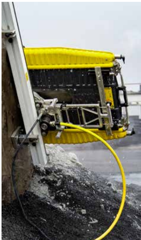
Unlike other manufacturers that cast their wall saw chassis, Pentruder machine mills its chassis from solid high-quality aluminum. This is to achieve the highest possible quality and durability and provides optimal weight distribution.
