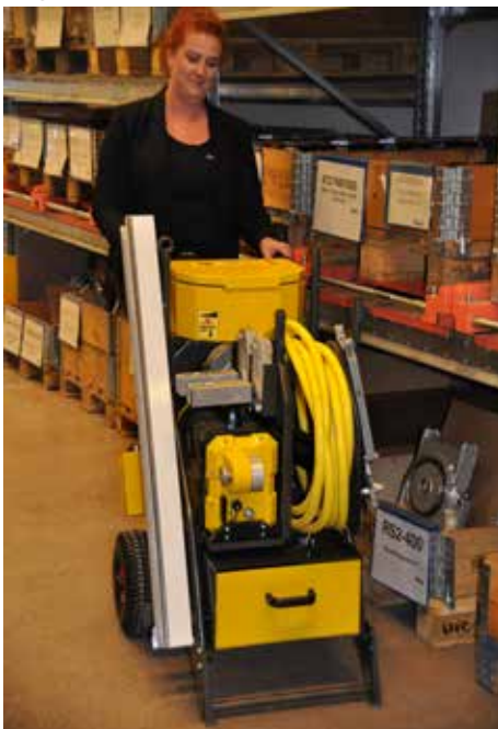
A flexible trolley that holds everything for the new RS2 wall saw. The blade guard is hung on the right side.
