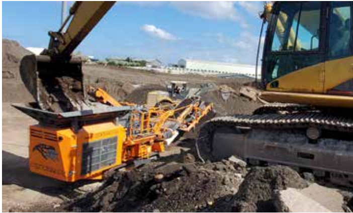
Currently, Alakona crushes about 5,000 tons a month with the R700S impactor.
