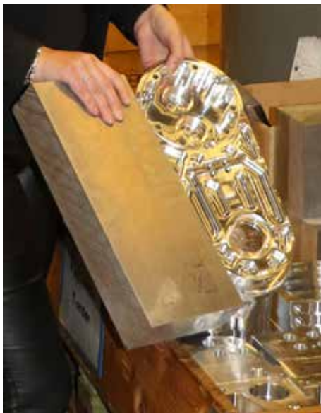
Unlike other manufacturers that cast their wall saw chassis, Pentruder machine mills its chassis from solid high-quality aluminum. This is to achieve the highest possible quality and durability and provides optimal weight distribution.
