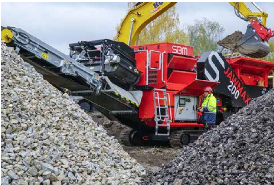
The new JAWMAX® 200 is the strongest lightweight in the compact class of mobile jaw crushers.
