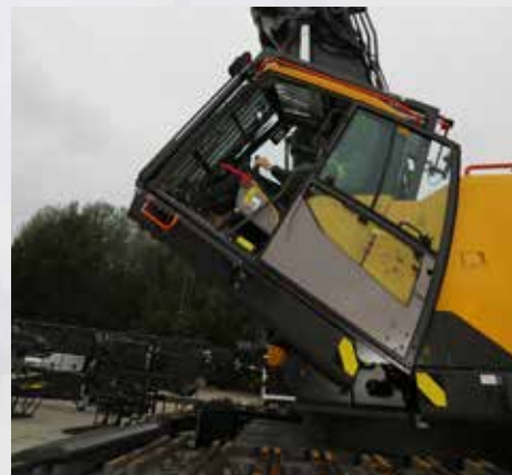
The cabin can be tilted up to 30°.
