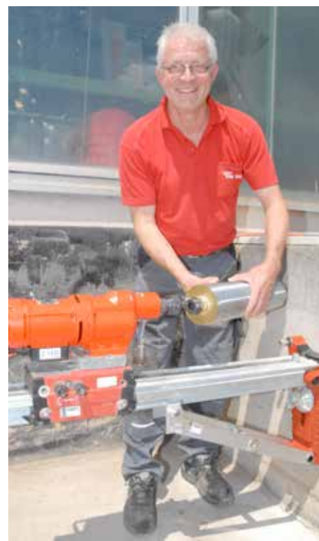
Dieter Steigerwald, workshop foreman at Betonbohrservice Findeis GmbH, mounts the drill bit on the drill motor with the tool-free PQ6 drill bit connection.
