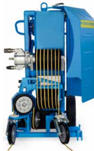
The hydraulic, ATEX-certified SB wire saw SB comes with up to 33 ft (10m) of wire storage, high power transfer thanks to multiple roller transfer and a hydraulic wire tensioner. Image © TYROLIT.
