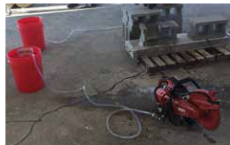
The DHS-P integrated water pump affords safe, convenient cutting.
