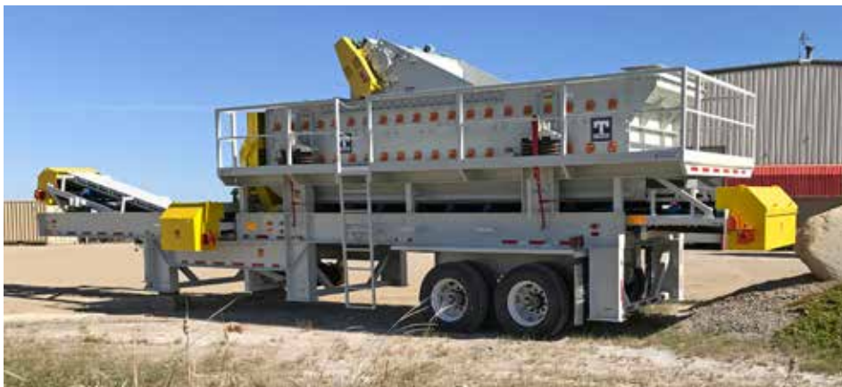
Haver & Boecker's Tyler L-Class vibrating screen is ideal for classifying wet or dry material or dewatering. The machine is easy to maintain with no timing belts or gears that normally need replacing. Image courtesy of Haver & Boecker.
