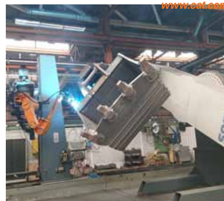
A new highly efficient welding robot at the Caterpillar plant in Den Bosch.
