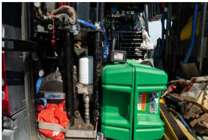
This HKR Hydraulic Screw Compressor is installed to the van, but it can be installed even tighter places too because the hydraulic oil flow provides cooling for the compressor.
