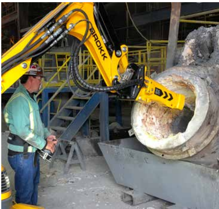
Brokk's heat-resistant features and remote operation increase productivity and safety for maintenance operations, such as ladle cleaning and refractory removal.
