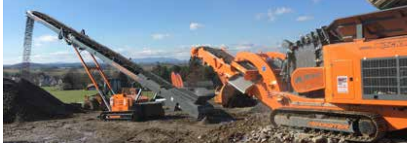
Processing concrete with the R900 impact crusher, and the RST 18 stacker.
