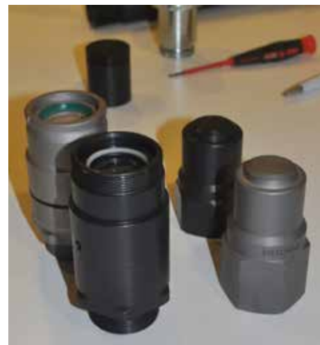
The new Qplus system includes a new sealing method that makes sealing exchange easy, increases oil flow which increases operational time.
