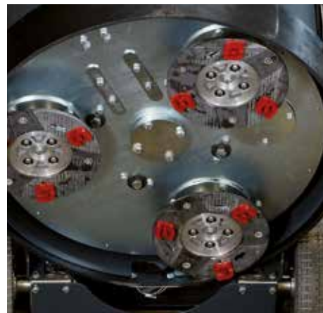
The grinding discs of the DSM 800RC were equipped with the new Giants SSC tooling.
