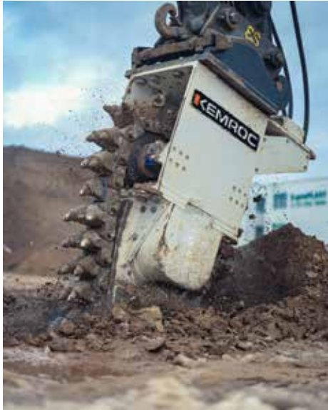
A major part of the KEMROC product range; the patented EK chain cutter attachments. One example is model EK 100, with moving cutter chains.
