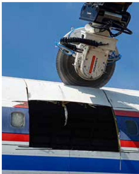
Sections of fuselage and other components were cut out. The cutting speed was equivalent to what would have been achieved using a conventional shearer.
