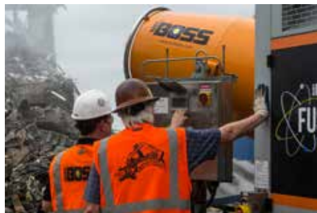
The mobile DustBoss DB-60 Fusion can be easily towed with a pickup or skid steer for repositioning.
