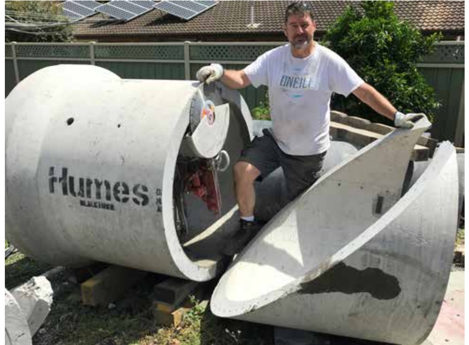
"This multi angle internal pipe saw is set to change the way pipes are cut," says inventor Paddy Brosnan.
