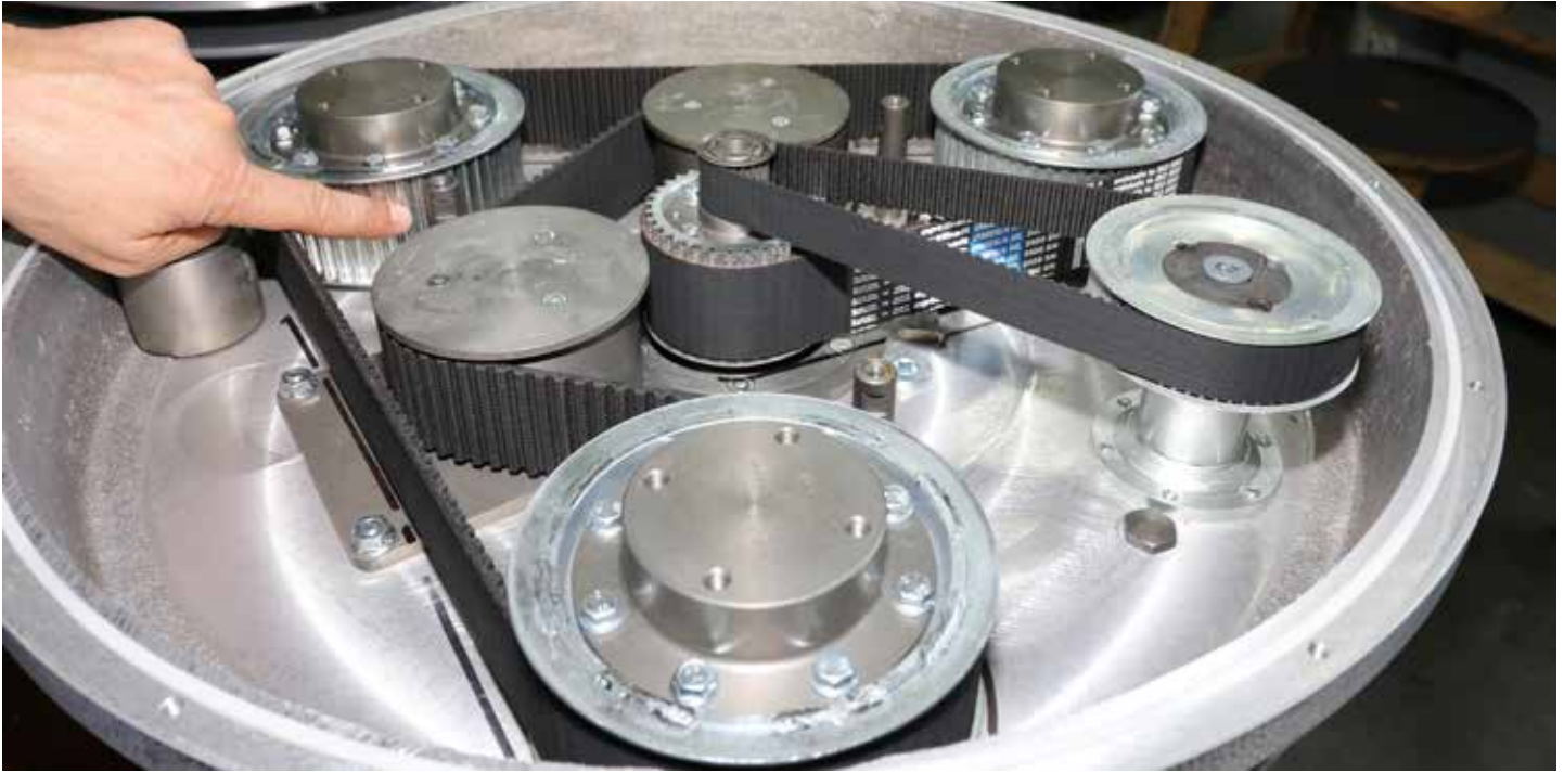
Lavina planetary grinding heads utilize timing belts. According to CEO George Popov, the timing belts are more durable and relatively easy to replace. The timing belt has teeth, which keeps it in place, and is superior to a poly-V and a flat belt, which might be slipping during operation.
