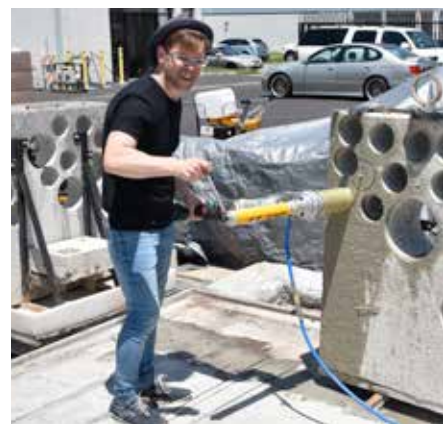
"The Core-EZ delivers cordless drilling in reinforced concrete with a 200mm core bit to the depth of up to 285mm, which is unmatched by the competing systems". PDA editor Andrei Bushmarin holding the core drill system.
