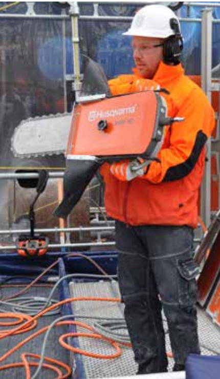
The new Husqvarna chain saw modul for wall saws to prevent overcuts.
