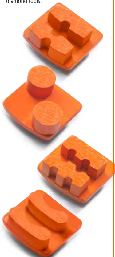
Redi Lock® G 1400 is a metal-bond diamond tool for very hard concrete. Each grit size has its own shape to be easily recognized. The shapes of the big (lower numbered) grit sizes are very aggressive and are to be used at the first steps. The shapes of the smaller (higher numbered) grit sizes are more round and smooth and are to be used at the last steps. The segments are here placed in grit size order from left to right, starting with the biggest grit size.
