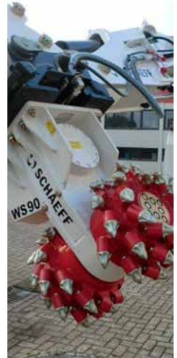
Above a cutting unit WS 90 mounted on the tunnel excavator TE 210.
