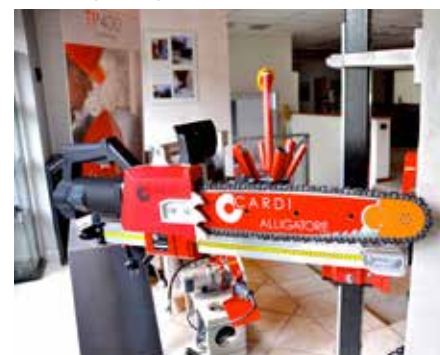
Cardi's chainsaw Alligator for masonry cutting.
