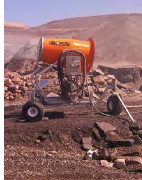
The company chose the DB-45 based on its range, able to throw the plume of atomized droplets 150 feet (45.7m) for effective dust control.
