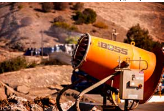
RAI has successfully employed an atomized mist system to suppress dust in and around its Chula Vista plant.
