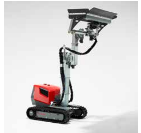
The new Aqua Cutter 410 has been designed for hydrodemolition applications in confined areas with restricted space. The boom can easily be manoeuvred in different position for optimal reach and removal of damaged concrete.
