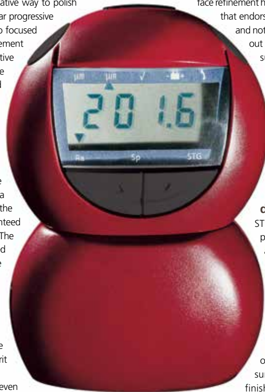
The T-Meter is electronically measuring the Ra, the STG and CSP (Concrete Surface Profile) 1-6 for floor preparation.
