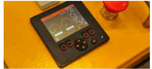
Conjet ONE makes controlling the robot much easier.
