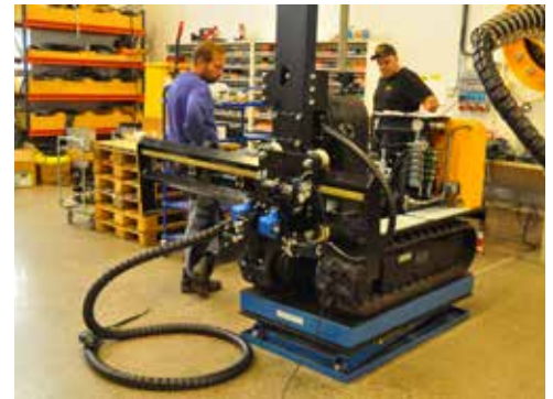
Above, the smallest hydrodemolition system on the market, Jetframe 101 Nalta, launched about three years ago.
