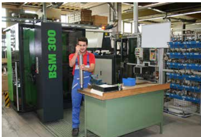
The Dr. Fritsch BSM 300 for laser welding core bits from from 3.5 inches to 12 inches (8 mm to 305 mm).
