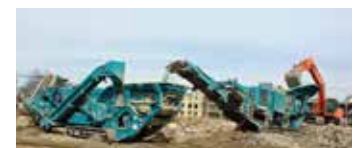
The Powerscreen XR400S primary jaw plant (right) and Powerscreen XH320SR impactor plant.
