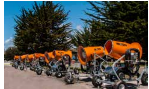
CalTrans rented eight DustBoss® DB-60s for dust suppression on the Doyle Drive project, with on-site training supplied by the manufacturer.
