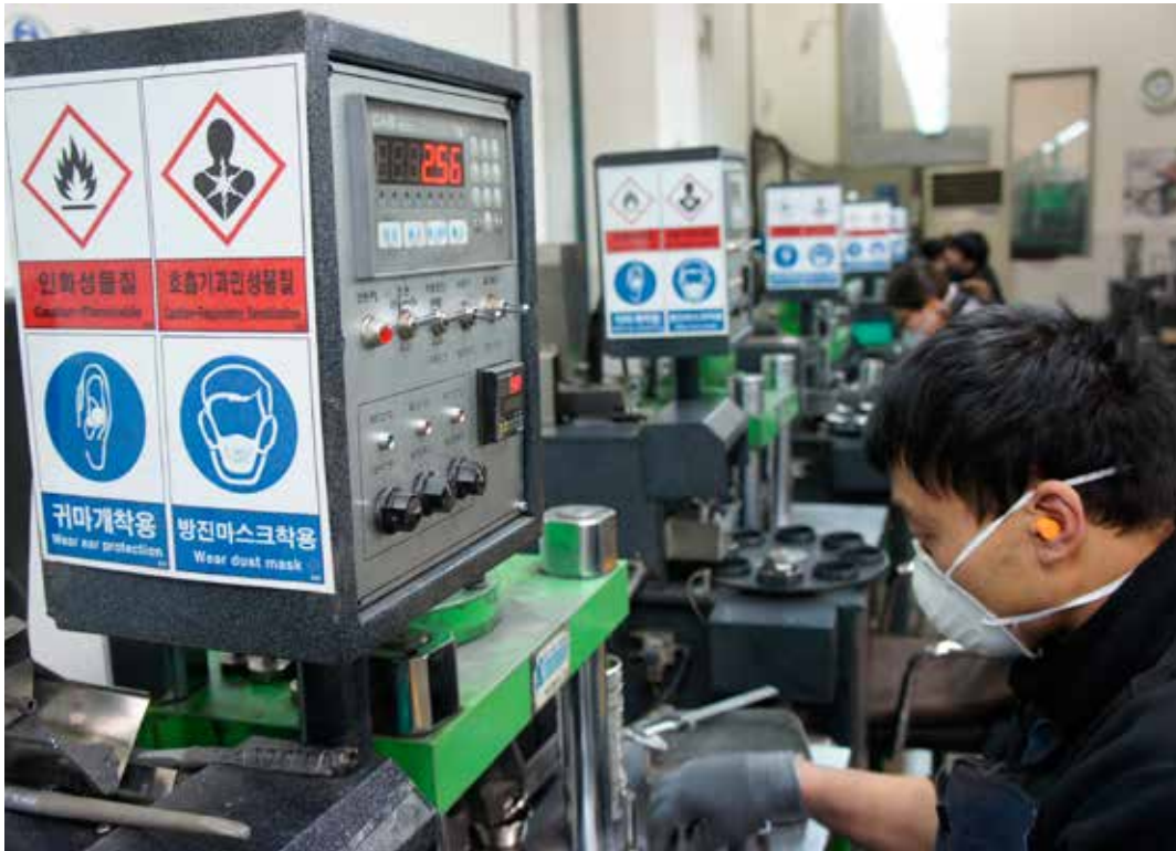
John Han has developed and built most of the automated manufacturing machines himself. This particular machine thread the beads automatically on the wire.
